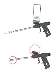
It is important to clean the gun after each use so that the excess adhesive does not render it unusable: screw the can of cleaner onto the gun and pull the trigger until there is no more adhesive inside. To avoid staining the floor, a simple way is to empty the excess adhesive onto kitchen paper placed in a waste paper basket, for example. It takes no more than 1 minute to clean the gun, then spray the gun socket where the can is placed, as well as the tip of the gun.
