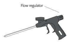
Ensure that the flow regulator is fully closed by locking the trigger.
